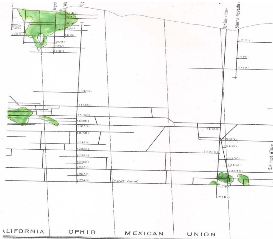
FIGURE 5 MIDDLE SECTION, COMSTOCK LODE, BECKER ATLAS SHEET X [BRACKETED FIGURES FROM SURVEYOR'S POINT AT A (GOULD & CURRY), CALIFORNIA EXHAUSTED AT 1,800' OPHIR (ORIGINAL DIGGINGS) AT 600', MEXICAN BARREN, UNION SMALL PATCH AT 2,600']
